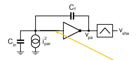
• We assume a perfect virtual ground at the amplifier input  $\rightarrow$  No charge can the go to C<sub>in</sub> (voltages are fixed)
