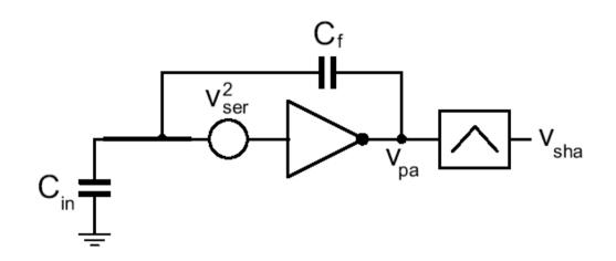
Output noise is determined by the capacitive divider made from C<sub>f</sub> and C<sub>in</sub>: v<sub>ser</sub> = v<sub>pa</sub> × Z<sub>Cin</sub> / (Z<sub>Cin</sub>+Z<sub>Cf</sub>)
