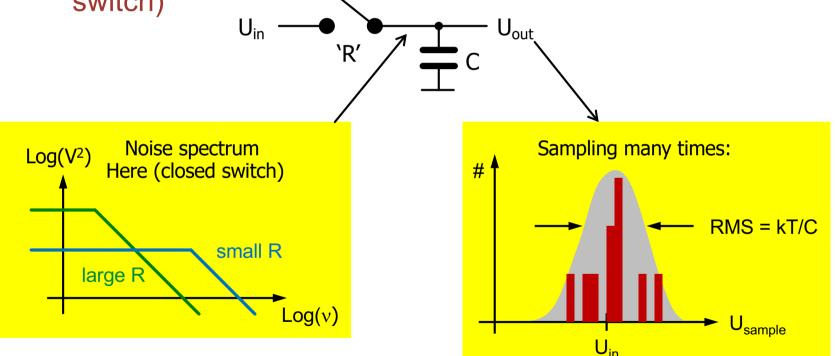
Precise sampling (voltage storage) needs large storage cap
