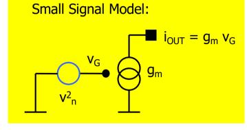
Due to input voltage noise source, we get at the output
