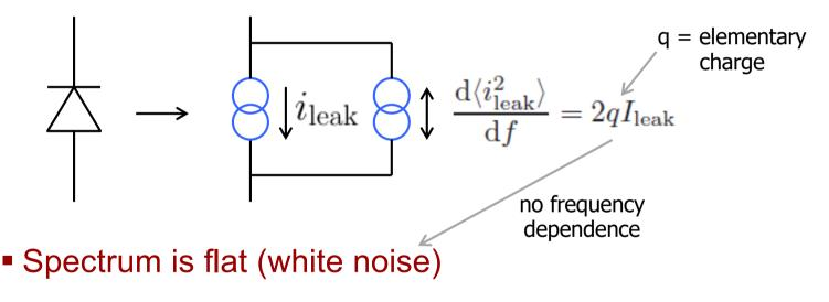
• Check the units:  $[2 q I_{Leak}] = C \times A = As \times A = A^2/Hz$
