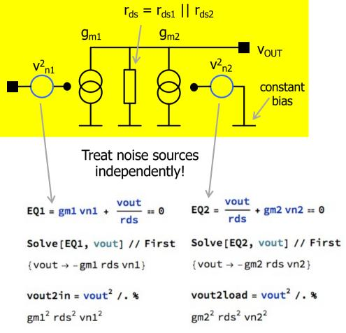
Input MOS must have high  $g_{m1}$ Bias Source must have low  $g_{m2}$
